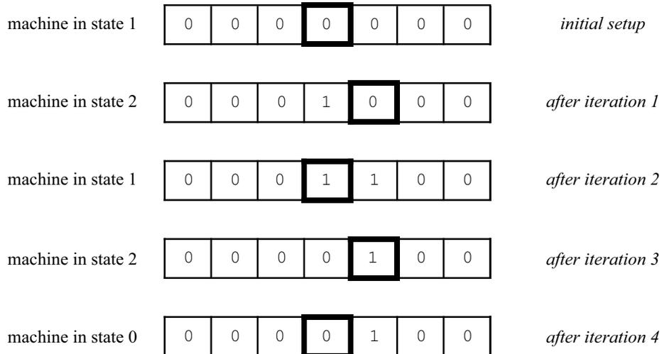
One instruction is processed on each iteration of the simulation until state 0 is reached. There are 4 iterations in the example simulation.
